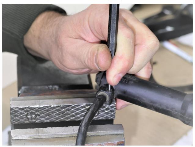
Remove and discard the line-end and quad-ring. You may keep the roll-pin and repurpose.
