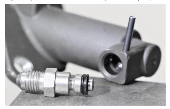
Install the replacement quad-ring on the fitting and lubricate with DOT 3 brake fluid.
